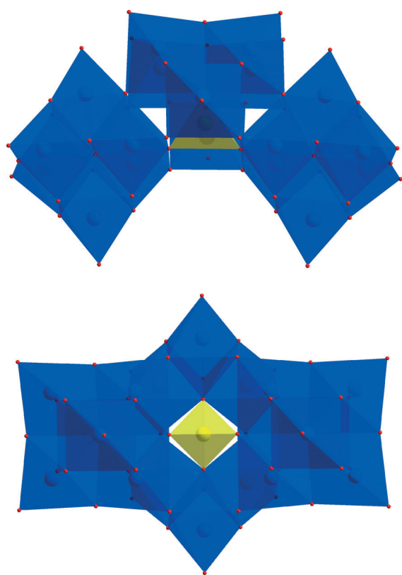
Figure 1. The structure of polyanion 1 in polyhedral representation; blue Nb, yellow Si, red oxygen.
